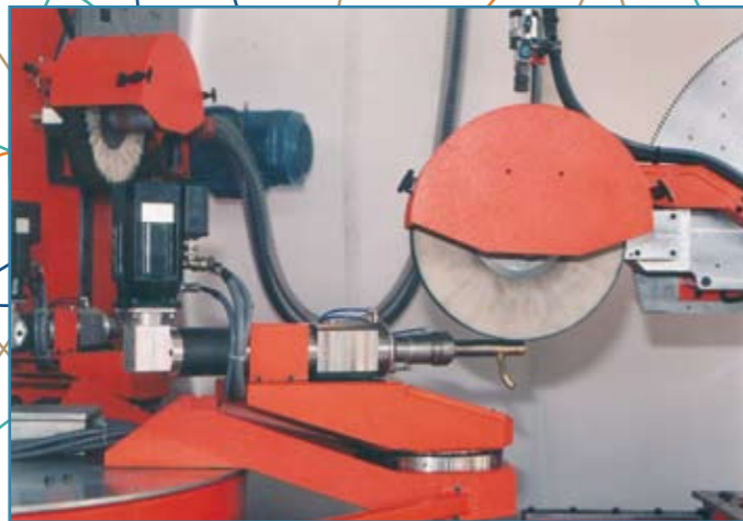
Polishing operation on taps/faucets
