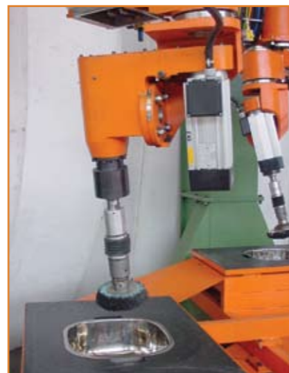
Polishing of sinks with ventilated buffs
